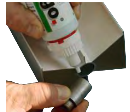
Application of an ergo. ® retaining compound on heating systems
